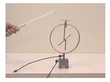
When a positively charged rod is brought close to the terminal, it pulls additional electrons out of the electroscope toward the terminal, rendering a greater positive charge on the electroscope, as seen.
