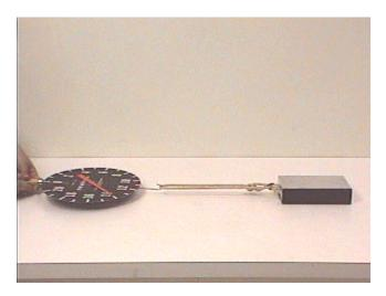
The coefficient of static friction is greater than the coefficient of kinetic, or sliding, friction. Therefore the greatest force is required to *start* the motion by overcoming the initially static friction. After the block is moving, the (kinetic) friction becomes less, so the force required to maintain the small but constant velocity becomes less, as can be seen in the video.
