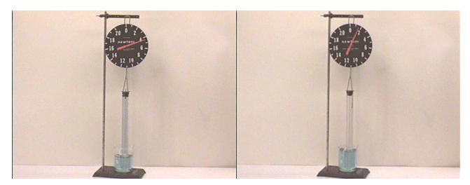
This may be a surprising result, considering that the water is held up in the tube by the force exerted by the atmosphere, and not by the spring scale. Now we must identify the force that changes so that the spring scale reading goes up.
