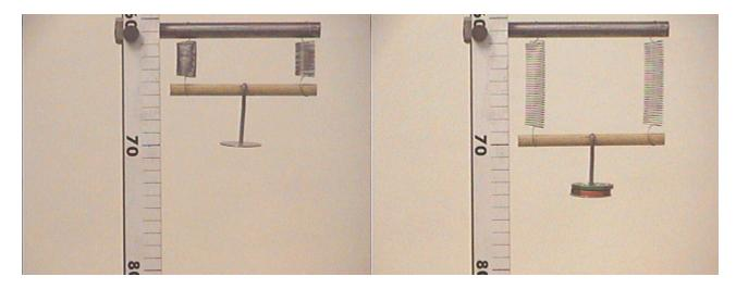
The downward force due to the two weights is shared between the two parallel springs, so that each spring feels the force of only one of the weights. Thus each spring is extended by 4 cm, so the location of the weight hanger will be 74 cm.
