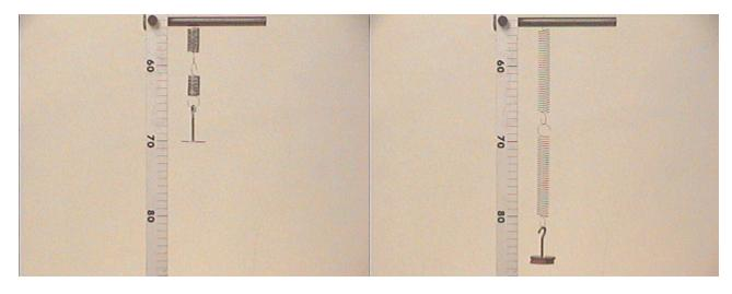
Note that the same weight is acting on both springs. According to the information provided for the single spring, the given weight causes each spring to extend by 8 cm, so the combination in series extends by twice that amount, or 16 cm. The end will be at 86 cm on the scale.
