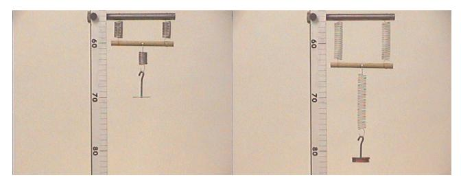
The entire weight hangs on the series spring, causing it to extend by 8 cm, while that weight is divided between the two parallel springs, causing them to extend by only 4 cm each. This is a total extension of 12 cm, so the position of the weight hanger will be 82 cm.
