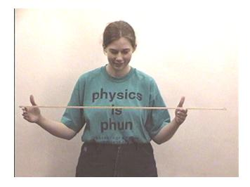
The finger closer to the center of the meter stick supports more of the weight, so that one has more frictional force with the meter stick and the other one slides. This continues until the sliding finger moves closer to the center, and the situation reverses. The two fingers alternately slide and stick until both fingers contact at the center.
