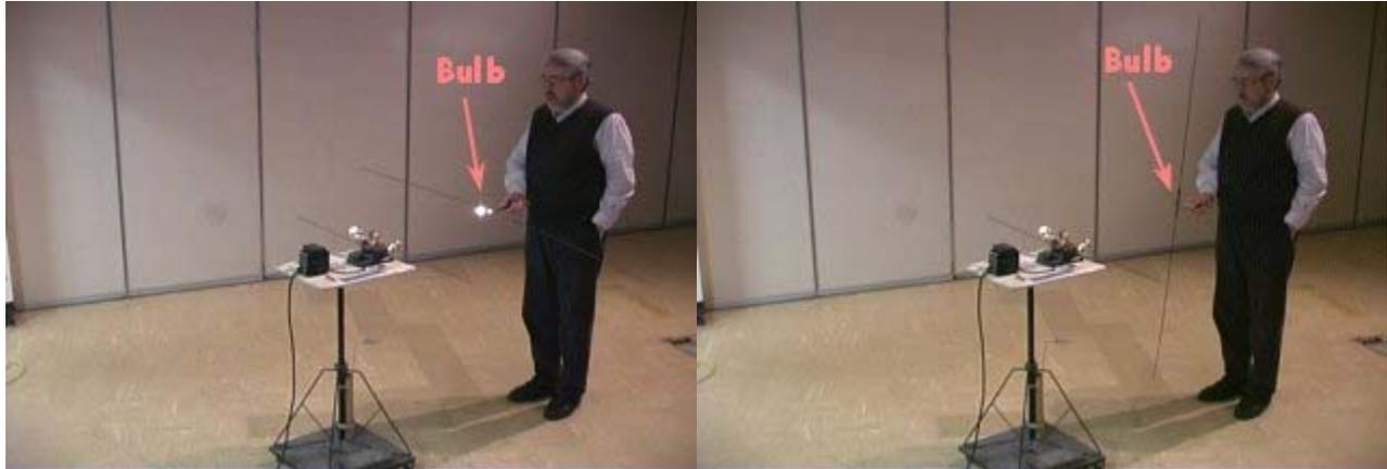
The waves from the transmitting antenna are polarized in the horizontal direction - the orientation of the antenna. A receiving antenna perpendicular to the receiving antenna will only send or receive vertically polarized waves, so the light will go out.
