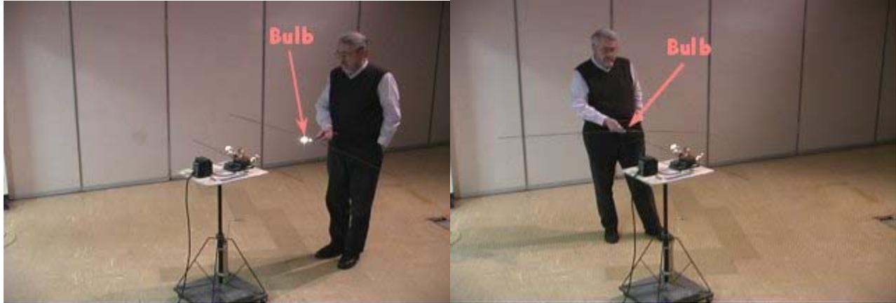
The waves from the transmitting antenna form a "dipole antenna pattern" in the horizontal plane with the maximum energy flowing away from the center of the antenna in a plane perpendicular to the antenna. There is a minimum of energy flow along the line of the antenna. This means that the "antenna pattern" of radio or TV stations may affect the direction in which the signal is larger or smaller, or may even result in the signal being so small that a station cannot be received.
