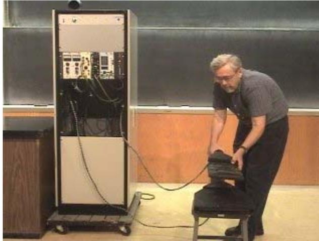
Secondary cosmic rays, such as the cosmic ray muons detected by these scintillators, originate from interaction of primary cosmic rays with atomic nuclei in the upper atmosphere, and move primarily nearly straight down from that point. This means that if the two paddles are directly above each other they will be more likely to have interactions with the same cosmic ray particle, creating more coincidences.
