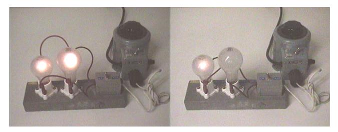
A small light bulb has more resistance than a large one, so that it will pass less current and consume less power:
