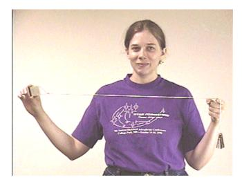
When the matchbook is released, it begins to fall, rotating about Gwen's finger on the string. As the keys fall, the string becomes shorter, leading the matchbook to rotate faster and eventually loop around her finger enough times that friction prevents the keys from pulling the string to the floor.
