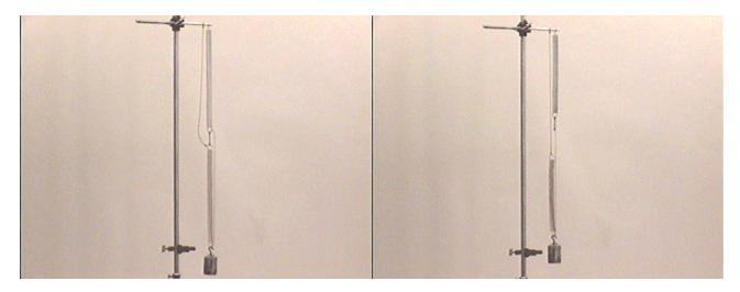
When the two springs are in series the entire weight is pulling on both springs. With the series/parallel setup each spring only supports half of the weight, and is therefore extended only half as much. The small amount of slack in the string cannot make up for the reduced spring extension, and the mass moves up.
