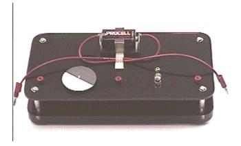
When the voltage is applied to the series system, the motor immediately starts. Note that when the motor is operating at high speed with little or no load it draws very little current. While there *is* current flowing through the series circuit, it is sufficient to keep the motor running but not sufficient to light the bulb.
