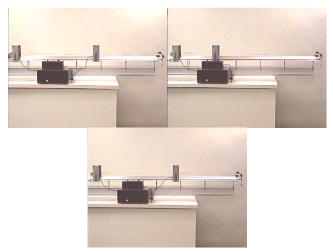
Releasing M allows m to accelerate it along the air track. The timer measures the time taken for a flag on the top of the air track glider to travel from photocell gate "A" to gate "B," which turns out to be exactly 2.00 seconds. See a video of the action by clicking your mouse on the photograph at the left above.
