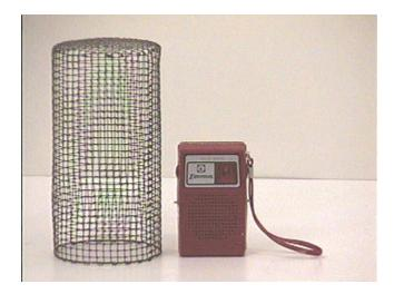
What happens to the sound of the radio after the wire mesh is in place.
