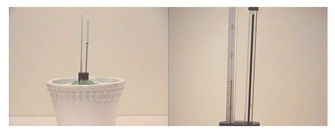
If the water in the flask were to expand, the green water level would rise higher into the capillary tube. On the other hand, if the water in the flask were to contract, the green water level would fall lower in the capillary tube. The flask used is made of quartz, which has a very small coefficient of thermal expansion, so if the flask and the water change temperature the predominant effect will be due to the expansion or contraction of the water.
