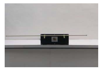
The meter stick is held in position as shown, and the motor driver started, causing the supports to rotate at a few revolutions per second in the sense shown in the figure below (forces inward on the meter stick), opposite to the case of Question #215.
