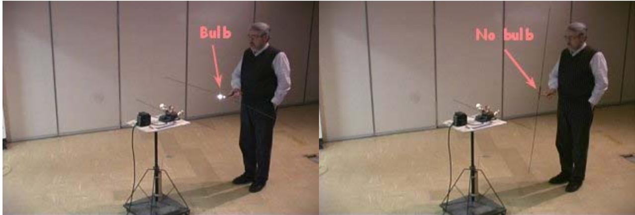
Now suppose that the light bulb is removed from the receiving antenna and it is rotated so that it is vertical, as seen in the photograph at the right.
