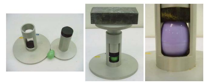
Now suppose that we put a *real egg* between the two rubber surfaces rather than a plastic egg. This situation is shown in the photograph at the left below, except that there are no lead bricks, only the weight of the plunger. At the right we see a close-up of the egg between the two rubber surfaces.
