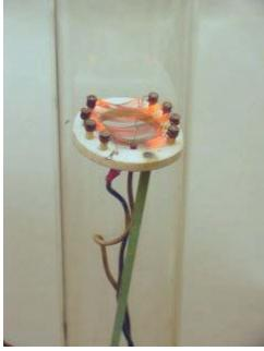
If we heat up the nichrome wire so that the Rijke tube emits its tone, then rotate the tube so that it is horizontal:
