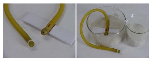
The hose, as seen in the upper left, is sealed on one end using a metal ball as a stopper. The other end is open, and a blast of air can be blown from the open end to the slit. The hose will be placed carefully in the dish and then buried with sand, with the slit facing up, as seen in the upper right.
