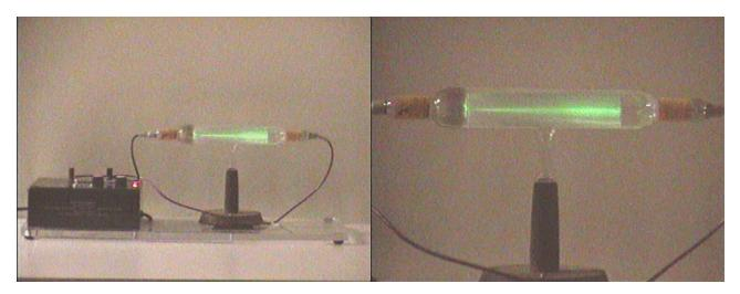
A bar magnet will now be moved close to the electron beam, with the North end of the magnet closest to the tube, so the magnetic field lines are pointed away from the viewer into the picture. What will happen to the path of the electron beam as the magnet is moved close to the tube?
