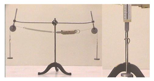
Now suppose that an identical 150-gram mass is supported from strings passing over pulleys, with an identical scale and a spring connected to the strings between the pulleys. This situation is seen in the photograph at the left above.
