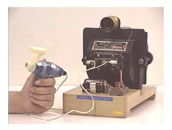
For this question we crank the generator, creating current in the inductor, then release the handle of the generator. What will the handle do - in particular, will it move, and if so in which direction?
