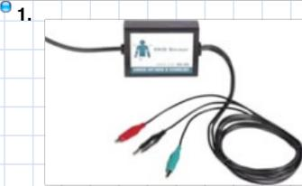
2. The EKG sensor plugs into one of the sockets on the left side of the LabPro. It has three alligator clips, colored red, black, and green.
