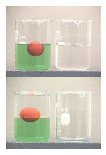
The ball floats at a higher level because the mineral spirits in which the upper part of the ball is floating provide an additional buoyant force on the ball. If the ball is floating on water alone, the top part of the ball is immersed in air, which has a much smaller density.
