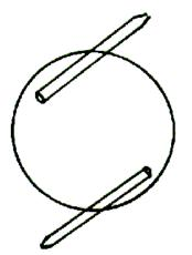
Now we solder the tubes to the can. Use a high wattage soldering gun or iron (the Radio Shack 100 watt soldering gun works great), since the can will absorb a lot of heat, and the little soldering pencils used for fine work in printed circuit boards aren't good for the kind of plumbing we are doing. Always use <u>lead-free solder</u> on any toy or object that will be handled, especially by children, who are more sensitive to lead poisoning.
