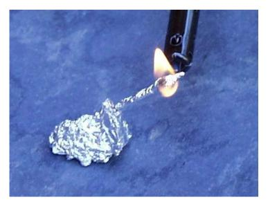
The heat of the flame will cause the matchhead to catch fire inside the foil. The hot gases from the matchhead will have only one way to escape -- through the hole where the pin is. As the gases go one way, the rocket goes the other, with a sharp hiss, and a trail of smoke.
