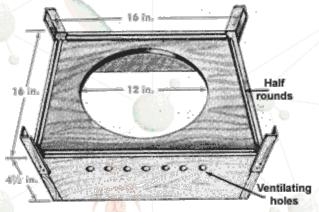
so that the masonite wall can be easily removed. Cut an app. 12" (30cm) hole in the top center. This hole needs to be the correct size to hold the pie pan, so use it to measure. Drill 7 1/2" (20cm) ventilating holes near the top of any two facing sides. You can fashion adjustable legs to the bottom (open) end if you wish.
