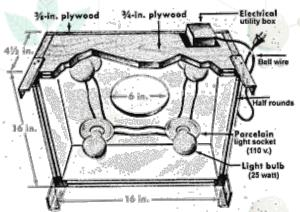
Assemble a box from 2 pieces each of the 16" and 14 1/2" 3/4"plywood, using a 16" square for the top. This is the top of the unit, and will orient so the open end is at the bottom. The finished box should be 16" (406mm) square. Cut a 6" (150mm) hole in the top for the
