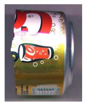
We then carefully (so as not to cut our fingers) bend over the sharp edge, and crimp it with a pair of pliers to form a neat edge. Don't worry too much about neatness, since it will not affect the operation of the engine, only the looks.
