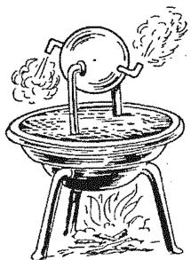
Hero's steam engine was probably a toy (if it was ever actually built) and not put to any useful purpose. Continuing in that fine tradition, we will build a version of his engine for the same purpose. Our version will be *much* simpler to build, since we will need no steam-proof bearings for an axle.
