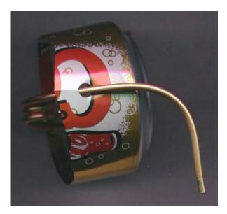
Next we bend the ends of the tubing gently so they curve into a right angle. Each end is bent opposite the other, so the can will spin when it is placed in the water and the engine started.
