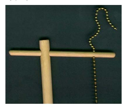
With the large dowel snug in the hole in the base, and the smaller dowel fitting in the hole near the top of the larger dowel, the chain now suspends the can a little above the base. Raise the chain enough to fit a small can of Sterno (jellied alcohol, used to keep food warm at buffets) under the Oatey can. Leave about a half of an inch between the two cans so air can get to the alcohol.
