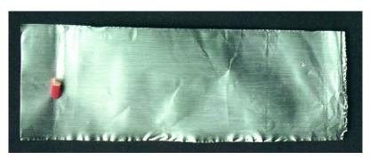
Roll the edge of the foil over the matchhead, forming a tube with the matchhead firmly in the center. Unfold the paper clip and insert one end of the wire into the tube so it touches the top of the matchhead (not the paper). Now press the foil tube flat to hold everything in place.
