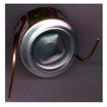
The final photograph shows the engine in operation. With a candle, it spins at about one rotation per second.
