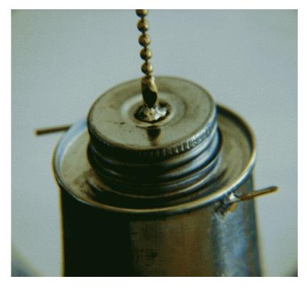
Next take the lid of the can and use it to trace a circle around some rubber sheet, either a piece of an old inner tube, or a bit from a tire patch kit. Cut out the circle and push it into the lid of the can as a seal (called a gasket) to keep the steam from coming out where it shouldn't.
