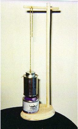
Now fill the can with water, tighten the lid firmly, and light the Sterno to boil the water in the steam engine. If the can is full of water it will take a few minutes to boil. If the can has only a half inch or so of water, it will boil much sooner. Be careful not to let the can run dry, or the can will become an ugly color, the solder will melt, and the rubber gasket will smoke and stink.
