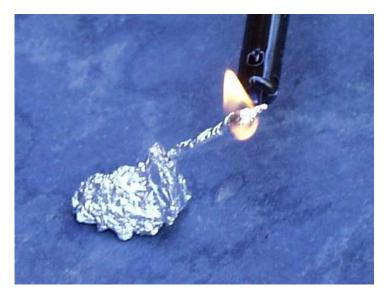
The heat of the flame will cause the matchhead to catch fire inside the foil. The hot gases from the matchhead will have only one way to escape -- through the hole where the pin is. As the gases go one way, the rocket goes the other, with a sharp hiss, and a trail of smoke.
