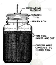
Press a strip of tinfoil smoothly around inside the jar, taking care to work out as many as possible of the air bubbles that may be trapped under it. The foil should extend from the bottom about two thirds of the way up inside. The wax, when hard, serves to hold the foil tightly to glass. It should not cover both sides of the foil, though what little runs out on the other side will do no harm. The outside of the jar is covered with foil in the same manner. The bottom of the jar is not covered.
