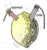
It is possible to get electricity from a lemon (and a few other acidic fruits and vegetables) using two strips of metal. The most readily available combination is copper and zinc. The zinc piece can be taken from the casing of an old carbon "D" cell (battery); some zinc coated nails may work as well. The copper can be a coin containing a high amount of copper. (Note: some recent copper coins, including the newer U.S. pennies, contain low amounts of copper mixed with zinc. If in doubt, use a pure
