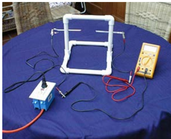
Ground Fault Interrupt box powering a hot dog cooker. Click image to enlarge.
