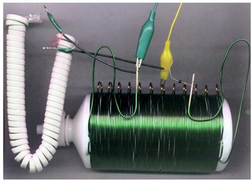
At this point, if all went well, you should be able to hear radio stations in the telephone handset. To select different stations, clip the alligator jumper to different taps on the coil. In some places, you will hear two or more stations at once. The longer the antenna is, the louder the signal will be. Also, the higher you can get the antenna the better.
