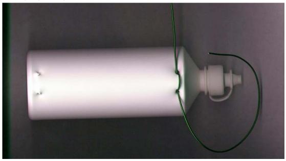
Now take the long end of the wire and start winding it neatly around the bottle. When you have wound five windings on the bottle, stop and make a little loop of wire that stands out from the bottle. Wrapping the wire around a nail or a pencil makes this easy.
