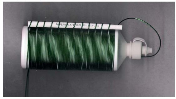
Cut the wire so that at least 8 inches remains, and thread this remaining wire through the two holes like we did at the top of the bottle. The bottle should now look like this:
