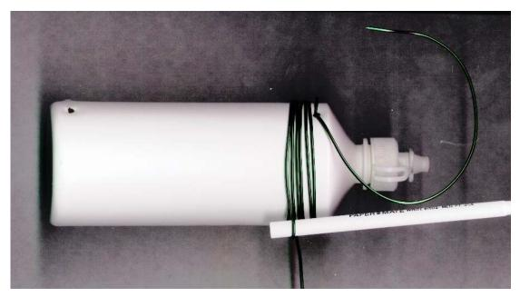
Continue winding another five turns, and another little loop. Keep doing this until the bottle is completely wrapped in wire, and you have reached the second set of holes at the bottom of the bottle.
