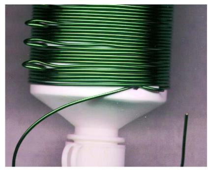
Now we remove the insulation from the tips of the wire, and from the small loops we made every 5 turns (these loops are called 'taps'). If you are using enameled wire, you can use sandpaper to remove the insulation. You can also use a strong paint remover on a small cloth,
