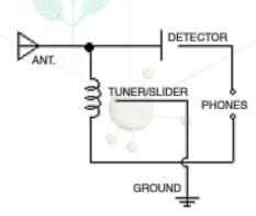
Refer to the schematic for wiring and connections. Wind the coil 100 turns around the tube. #22 AWG wire is recommended, but it is likely that whoever was in the field used whatever gauge was in the scrap coil, motor, or transformer they were cannibalizing. Spray / paint the coil with lacquer (or whatever is handy) to set it firmly. Scrape off whatever paint or varnish may be on the wire used for the tuner/slider. Spread the safety pin
