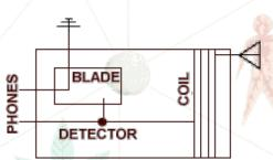
From what I can tell, there would have been only 3 terminals, one securing the antenna wire and one end of the coil; one with the detector (bent safety pin head) and one of the headphone wires; and one with the razorblade, ground wire and the other headphone lead. I have not built one of these. This
