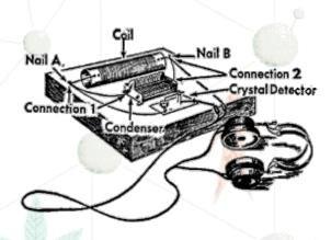
The antenna attaches to the nail that connects with the coil and razor blade (A). The ground wire attaches to the other nail, where the coil connects with the earphones (B). Hook up the headphones,
