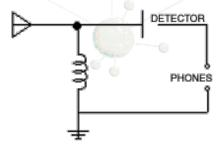
Not much can be said about so simple a design. The coil was 120 turns around a 2" form (toilet paper tube). The whole thing was tacked down to a board. Pencil lead wasn't used at the time, instead the safety pin point directly contacted the blue (or rusty) razorblade. There is no tuner, of course, so only one signal will be received, and only if there is a station broadcasting near the correct
