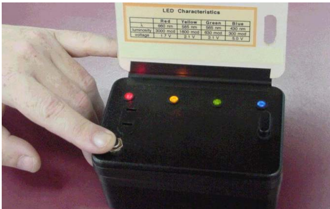
Fig. 3: This is a photo of the box with its lid open and its LEDs activated. The chart shows the peak wavelength, nominal luminosity, and operating voltage of each LED. The data were obtained from the manufacturer's LED packaging.
