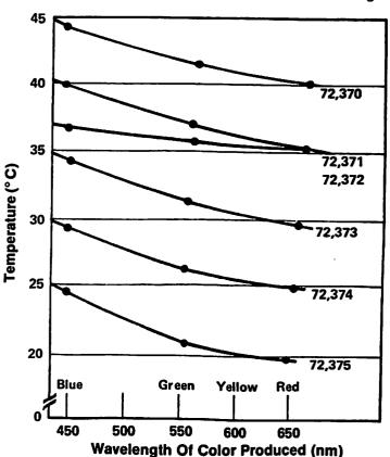
indicating a different temperature. Rubber cement, thinly applied to the test subject, will insure reasonably good contact. This technique, however, should not be used if the film is to be reused on other objects. Removal could cause separation of the LC from the plastic sheet and make it ineffective for further use.
