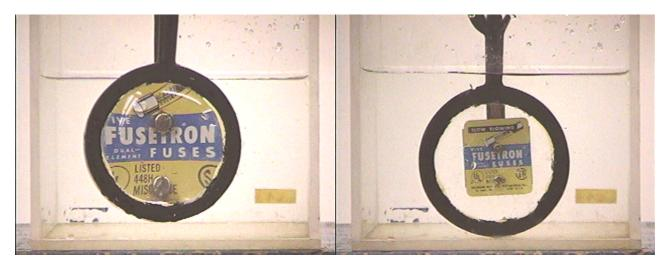
When the lens is immersed in water it no longer attains its normal focal strength, because the medium in which it is immersed has an index of refraction nearly equal to that of the glass in the lens. Light rays no longer bend as much at the interfaces where they enter and exit the lens.
