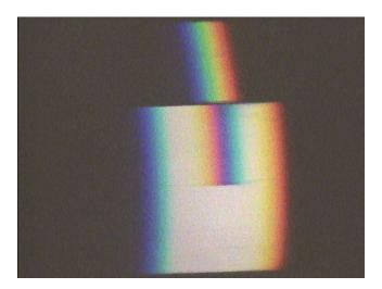
From the difference between the center and the lower spectra, the effect of the "negative" slit is apparent. Aberration in the optical system causes curvature of the spectra in this case, but does not affect the result.
