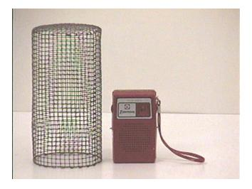
The wire mesh acts as a *Faraday cage* for the radio waves, stopping the radio waves from entering the cage and getting to the radio. This mesh will be effective for all radio waves with wavelength somewhat longer than the spacing of the mesh.
