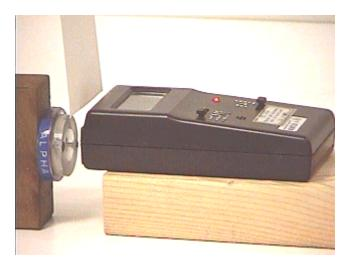
The <sup>237</sup>Am (americium) source produces alphas with about 5.5 MeV of kinetic energy. It only takes a sheet of paper to stop alpha particles from any naturally occurring radioactive material.
