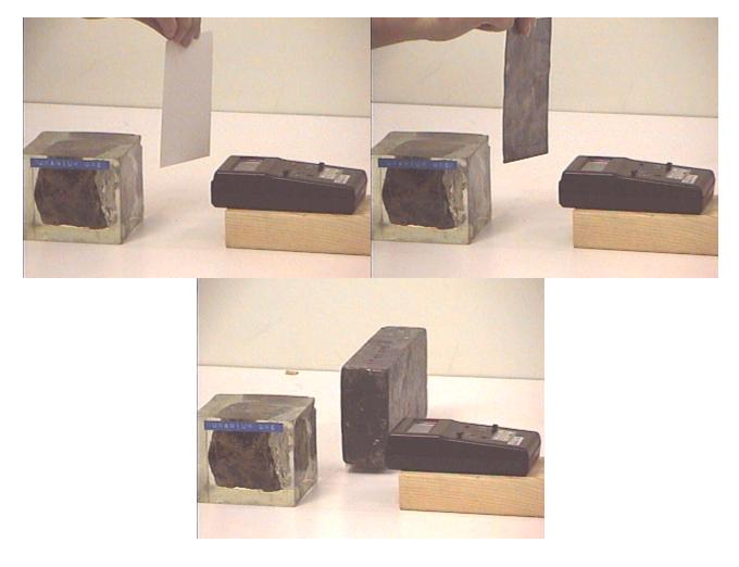
This source produces gammas with kinetic energy mostly less than 2 MeV, but surprisingly they have much more range, or penetrating ability, than the same energy of betas or much higher alphas. It may take the thickness of more than one lead brick to stop gamma rays from some naturally radioactive materials or from radioactive waste.
