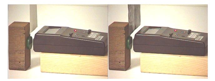
The  ${}^{90}$ Sr (strontium) source produces betas with a maximum kinetic energy of about 1.5 MeV. It takes a few millimeters of lead sheet to stop betas from most naturally radioactive materials.
