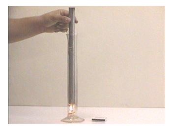
The tube serves the useful purpose of allowing the hot combustion products to rise out of the graduated cylinder and be lost in the surrounding atmosphere. When the tube is removed, the convection process (air coming down outside the tube and leaving up the tube) is impeded. The necessary oxygen in the tube mixes with the combustion products until there is not enough oxygen left to support the flame and it ceases. It only takes seconds!
