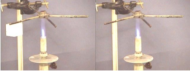
After the burner was lit (upper left) the copper wax fell off (upper right), followed by the aluminum (lower left) and the brass (lower right). This means that the thermal conductivity of copper is the greatest, aluminum is next, and brass is the least.
