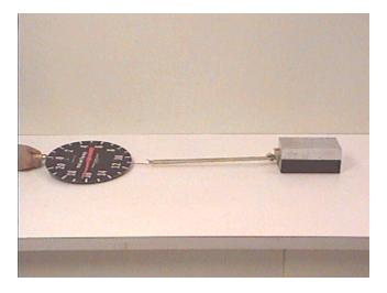
According to the "laws of friction," the frictional force between two surfaces is proportional to the normal force. When the normal force doubles (two blocks rather than one) the frictional force doubles, as it does here reasonably accurately.
