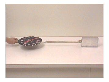
According to the "laws of friction," the frictional force between two surfaces with the same types of materials is independent of contact area, and dependent only on the normal force. This is very nearly the case here; the frictional force is only slightly higher when the smaller contact area is used.
