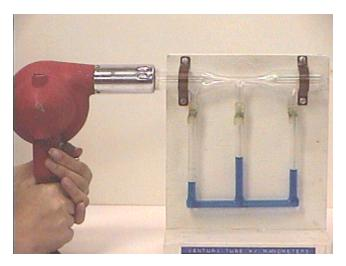
Two effects are present here. First, the pressure is dropping along the tube, so in the absence of the venturi constriction the water column would become higher from left to right. In addition, the constriction results in an increase in the speed of the air and a concommitant decrease in pressure, as seen in the photograph and the video.
