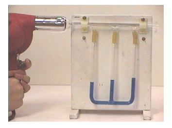
There is a pressure loss along the tube in any situation in which a fluid is flowing, for example, water in a city water distribution system or air in a tube as in this problem.
