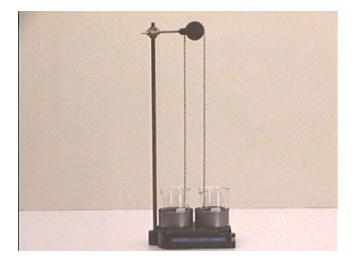
When a beaker is lifted, the weight of the chain on that side becomes less than the weight on the other side. Therefore the heavier side will pull the lighter side over the pulley.
