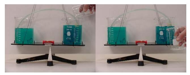
Note that the water level in the beaker at the right on the balance is higher than in the beaker at the left. The siphon will allow the water from the higher level to move to the lower level, causing the system to return to equilibrium.
