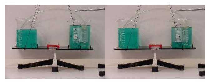
Note that the water level in the beaker at the right on the balance is higher than in the beaker at the left immediately after the aluminum cylinder is submerged, as seen in the photograph at the left. The siphon will allow the water from the higher level to move to the lower level, causing the system to return to equilibrium, as seen in the photograph at the right. It does not matter whether the entire cylinder or only part of it are submerged; in either case the water level will equalize.
